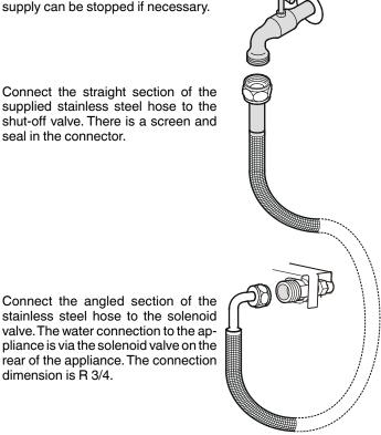
Before the appliance is used for the first time the system must be bled of any air by a competent person (i.e. Plumber)
