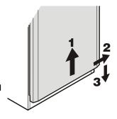
Tilt door inwards from the left 1. Secure hinge pin with screw 2.
