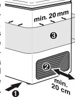
• Standard EN 378 specifies that the room in which you install your appliance must have a volume of 1 m³ per 8 g of R 600a refrigerant used in the appliance, so as to avoid the formation of inflammable gas/air mixtures in the room where the appliance is located in the event of a leak in the refrigerant circuit. The quantity of refrigerant used in your appliance is indicated on the type plate.
