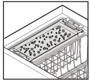
The freezer tray can either be suspended on the basket or can be slid into the interior container and used as a partition (except model GT 1456).
