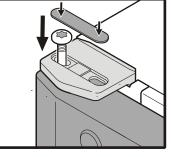
**16.** Tighten the torque rod with the open-ended spanner provided. > **60**°
